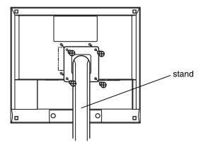
4 Mounting Screws (enclosed): M4 x 12 mm
